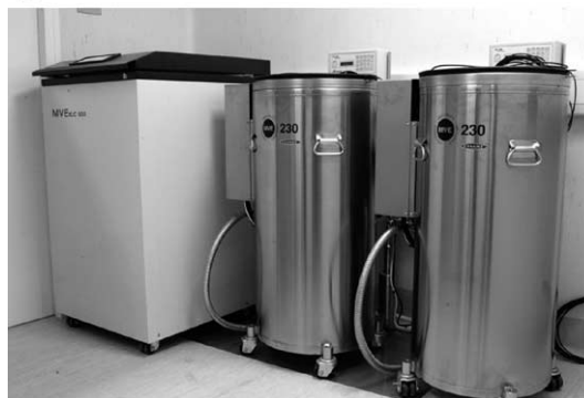
Fig. 2. Equipment in the UKSCB: (A) one of the three clean-room laboratories. (B) Liquid nitrogen storage vessels for the banking of the stem cell lines.
